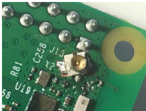
Figure 24: Soldering a IPX U.FL connector on the Raspberry pi 3. to extend it with an external WiFi antenna
